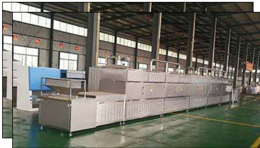
Figure 3 Microwave drying system for ceramic tiles [21]
